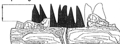
Figure 15 - Correct Flame Pattern With Control Knob Set to High Flame
