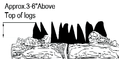
Figure 20-Correct Flame Pattern with Control Knob Set to High Flame
