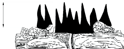
Figure 21 -Incorrect Flame Pattern with Control Knob Set to High Flame
