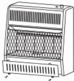
Figure 7 - Removing Lower Front Panel Of Heater
