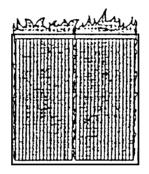
Figure 26 - Incorrect Burner Flame Pattern
