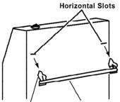
Stand-Out Tab Mounting Bracket (attached to wall)
