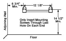
Figure 7 - Mounting Bracket Clearances
