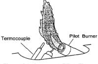
Figure 24 - Incorrect Pilot Flame Pattern
