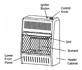
Figure1-Vent-Free Natural Gas Heater
