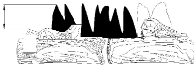
Figure 19 - Correct Flame Pattern With Control Knob Set to High Flame
