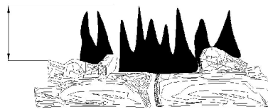
Figure 20 - Incorrect Flame Pattern With Control Knob Set to High Flame
