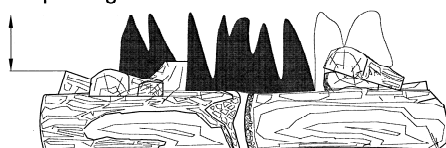
Figure 17- Correct Flame Pattern with Control Knob Set to High Flame (5)
