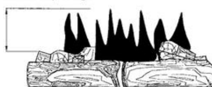
Figure 18 - Incorrect Flame Pattern with Control Knob Set to High Flame (5)
