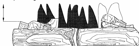
Figure 24- Correct Flame Pattern with Control Knob Set to High Flame (5)
