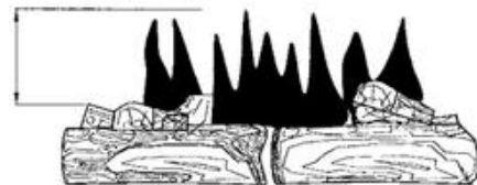
Figure 25 - Incorrect Flame Pattern with Control Knob Set to High Flame (5)
