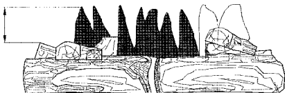
Figure 14 -Correct Flame Pattern with Control Knob Set to High Flame More Than 8" Above Top of logs
