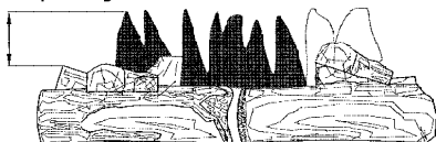
Figure 13 -Correct Flame Pattern with Control Knob Set to High Flame
