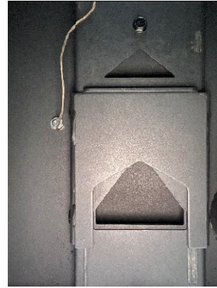
Air control mid-point setting for medium burn rate pulled by 1 inch from minimum setting
