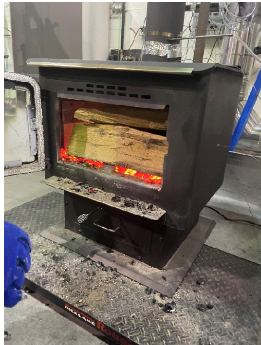
Low burn load in the firebox
