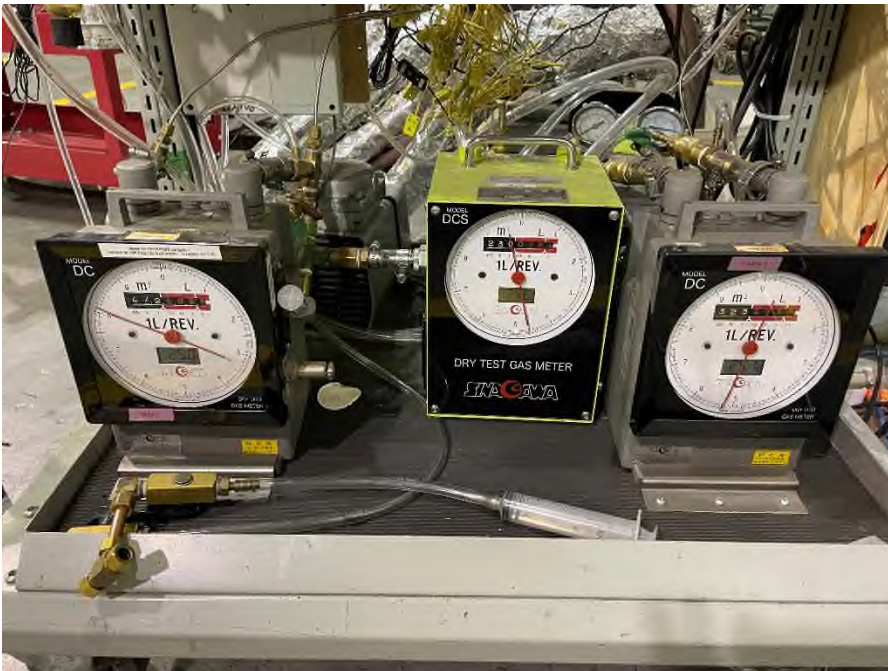
Picture 11: Dry gas meter
