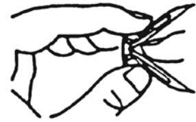
Fig. 17 - Folding the Expansion Bracket
