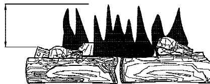
Figure 16 -Incorrect Flame Pattern
