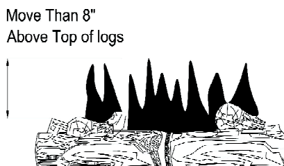
Figure 20 -Incorrect Flame Pattern with Control Knob Set to High Flame
