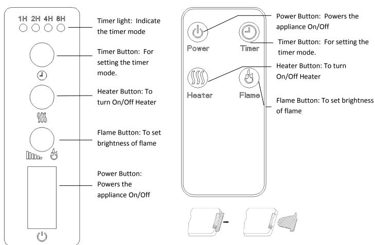
Pull the insulating film out of battery cover before using the remote control.
