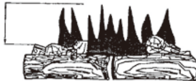
Figure 20 - Incorrect Flame Pattern with heater set to High Flame
