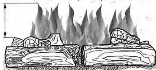
Figure 28 - Incorrect Burner Flame Pattern
