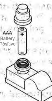
Figure 17 - Installing Battery in Ignitor
