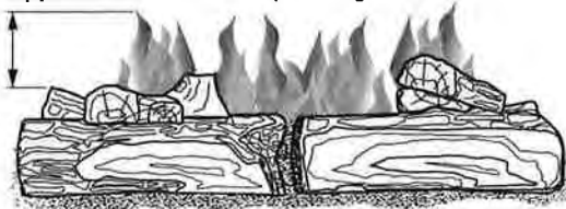
Figure 27 - Correct Burner Flame Pattern
