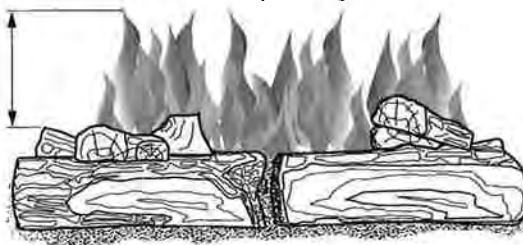
Figure 33 - Incorrect Burner Flame Pattern
