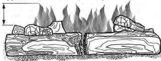
Figure 32 - Correct Burner Flame Pattern
