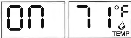
Figure 28 - Manual Mode in ON Operation
