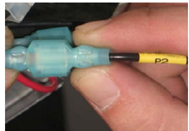
Figure 6 Insert the male port, which is on the black power supply wire (marked with P2), into the corresponding female port (marked with P2).
