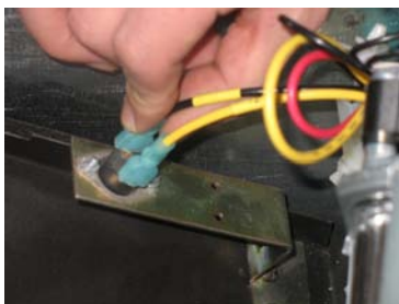
Figure 7 Connect two wires' female ports marked with T1 and T2 (black and yellow) with two male ports on temperature sensor.
