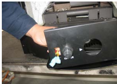
Figure 14 Pull AUTO, OFF, MAN wires from the hole of rocker switch.
