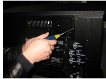
Figure 21 Check the safety of wires, and fix Blower Access Panel to back board.
