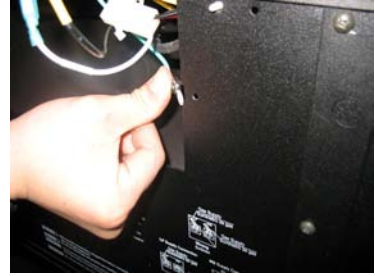
Figure 12 Push grounding slice to make its angle with back board more than 60°.
