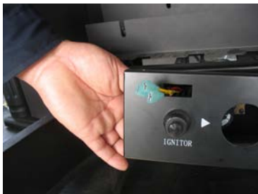
Figure 16 Pull AUTO, OFF, MAN wires from the hole of rocker switch.
