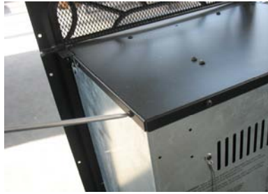
Figure 20 Fix the top panel with screws.
