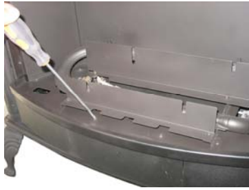
Figure 19 Re-fix Control Panel.
