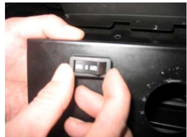
Figure 18 Push Roker Switch into Control Panel and fix it.
