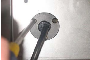
Figure 2 Fix the power cord, which are matched with metal wafer, to the top panel with three screws.
