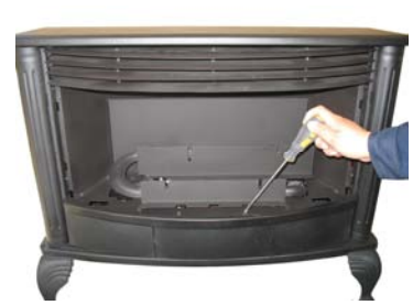
Figure 15 Unscrew screws for fixing Control Panel.
