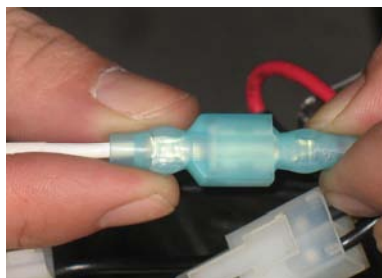
Figure 8 Insert the female port, which is on the white power supply wire (marked with P1), into the corresponding male port (marked with P1).
