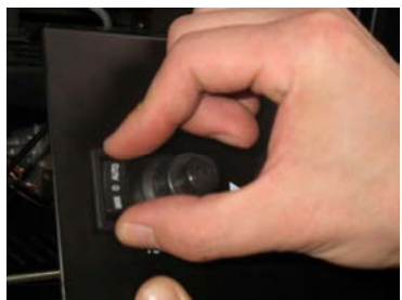
Figure 16 Push Rocker Switch into Control Panel and fix it.
