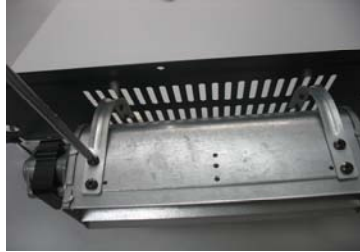
Figure 2 Mount Blower onto Blower Access Panel.
